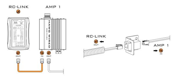
2. MULTIPLE AMPLIFIER CONFIGURATIONS: CONNECT YOUR AMPLIFIERS TOGETHER USING THE SUPPLIED FLAT LINK CABLES IN THE ORDER IN WHICH YOU WANT THE AMPLIFIERS TO BE SELECTED BY THE REMOTE. NOTE THE IN AND OUT PORTS OF EACH AMPLIFIER, AND CONNECT THEM ACCORDING TO THE DIAGRAM BELOW.
